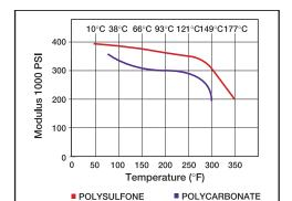
Fig. 16 - FLEXURAL MODULUS VS. TEMPERATURE
